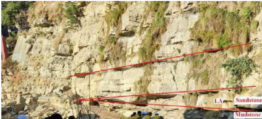
Figure 2: Photograph showing inter-bedding of thin mudstone and thick sandstone at right bank of Chidiya Khola, upper part of Lower Siwalik.
